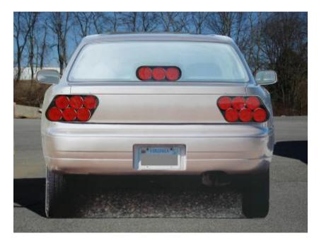
Figure 5. Vehicle Mock-Up with Working Brake Lamps
