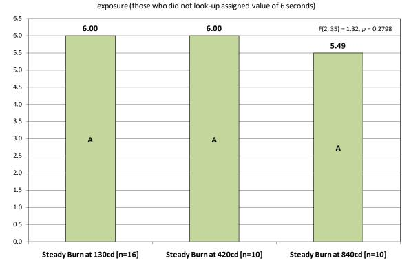
Mean Eye-Drawing Latencies By Steady-Burn Lighting Configuration, 1st Exposure Values represent latency to look-up from onset of emergency braking; glances for the 1st
